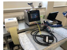
Images of AquaTYPHOON™ (left) in the pre-cleaning area and PlasmaTYPHOON+ (right) in clean area of the endoscopy decontamination unit
