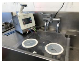
Images of AquaTYPHOON™ (left) in the pre-cleaning area and PlasmaTYPHOON+ (right) in clean area of the endoscopy decontamination unit
